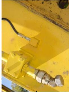
Steel Junction Block is welded to the side of the stick usually where the hammer hydraulic circuit is disconnected for quick removal of tool.
