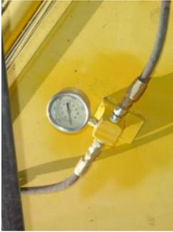
A pressure gauge bracket is welded on the cab side of the boom in view of the operator to confirm that the system is working properly. If there is no pressure reading while the hammer is operating, this indicates a problem with the system.
